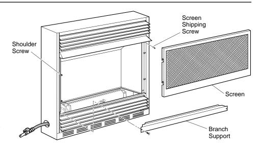
Figure 23 - Removing Branch Support From Fireplace
